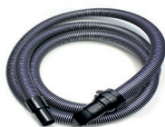
Suction hose grey/black, antistatic Ø 38 mm (1 1/2") L 5 m (16 1/2") complete with connecting pieces
